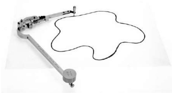
Above: Amsler Type 2 Polar Planimeter, Sold by Crosby Steam Gage & Valve, 1880s. Courtesy of the Smithsonian Institution's National Museum of American History.
