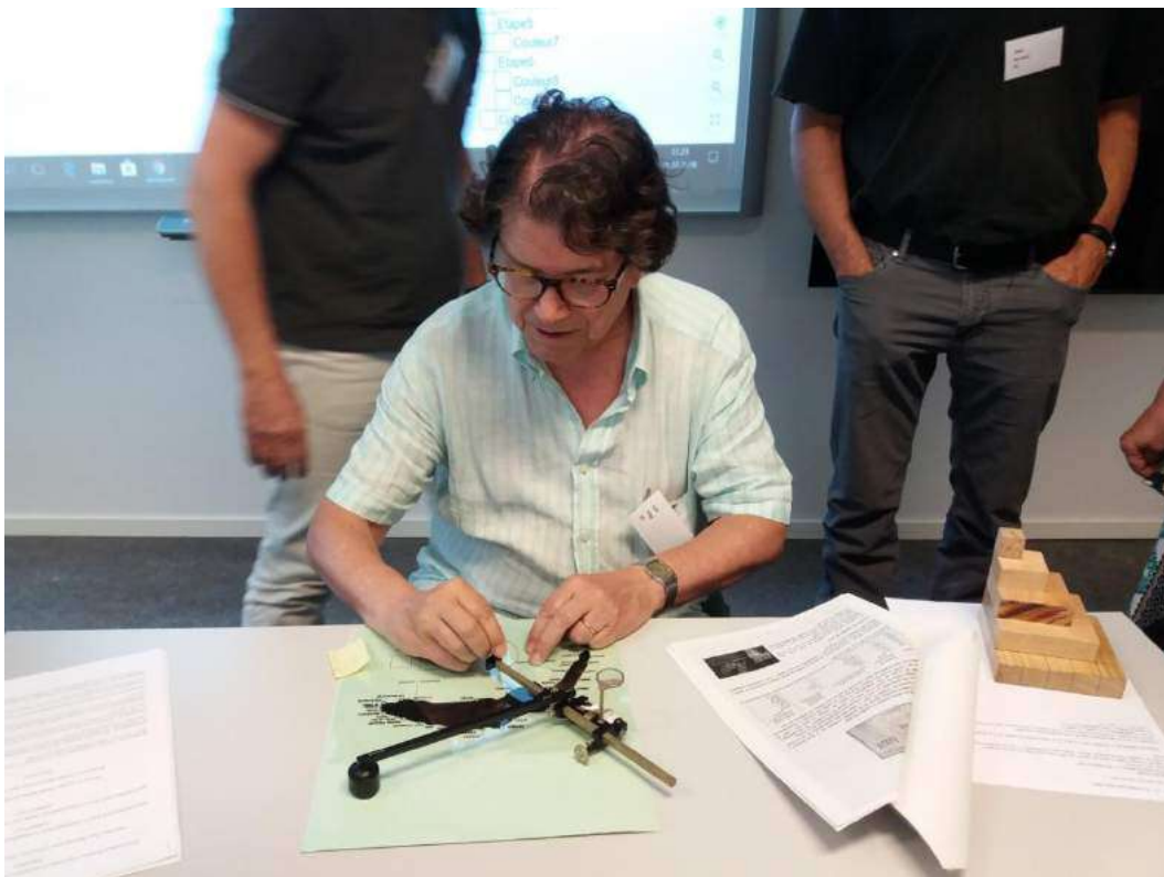
Picture 4.7: Using Polar Planimeter at the workshop
