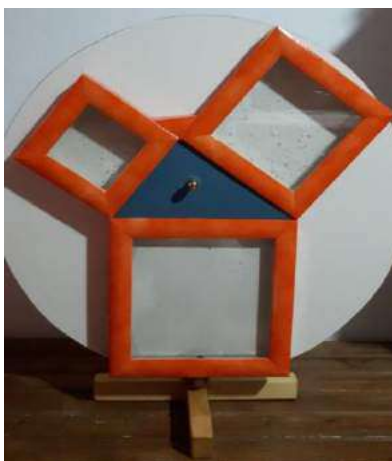
Figure 3.1: Hydraulic artifact to prove the Pythagorean Theorem
